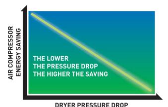
Poorly constructed heat exchangers and liquid separators create a high pressure differential across the dryer which leads to high operational costs and poor dewpoint performance.
