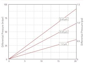
Flow (L / min) for liquid @ 20 °C and 1 cp 10"module Recommended wine flow rate of 4.5-10 I/min/10"module
